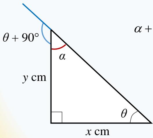
$$\alpha + \theta + 90^\circ = 180^\circ ; \quad \tan \theta = \frac{y}{x} ; \quad \tan \alpha = \frac{x}{y}$$
